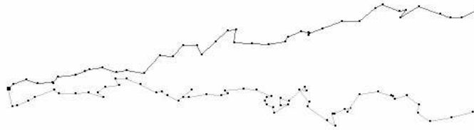
Fig. 2. Sample long-term behaviour of the BCI mouse with a fragment of data from the training set (top trace) and the validation set (bottom trace). Every dot in the plots corresponds to a motion vector issued by the system.
