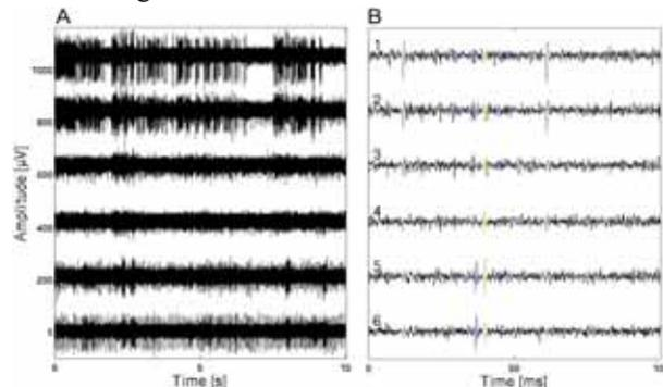
**Fig. 2. (A)** | Recordings from *rd1* mouse retinal ganglion cells. **(B)** | Zoom into (A) with spikes from 3 units identified after spike sorting and marked in different colors. Note: each unit is detectable on more than one electrode.
