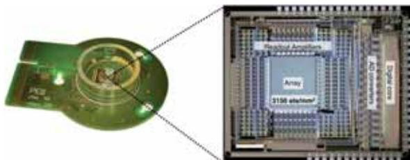
**Fig. 1.** Packaged high-density MEA device and overall chip micrograph. Scale bar: 1 mm.
