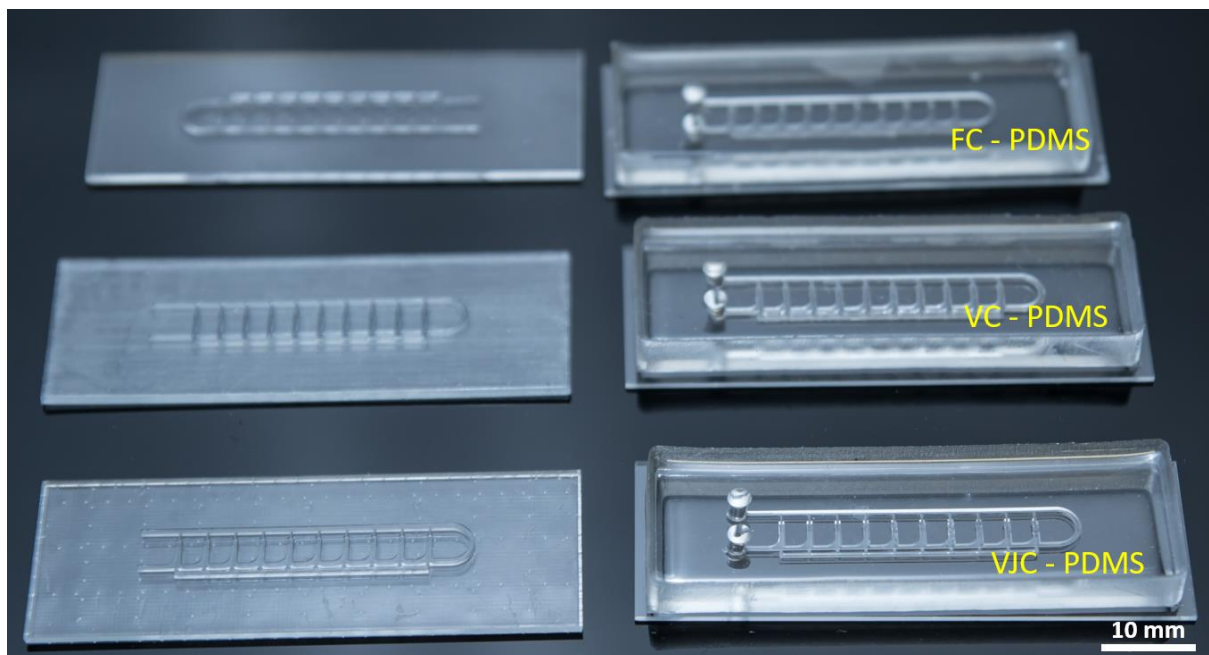
Figure 5.4 A photograph of 3D printed mould and the final fabricated PDMS chip-based device. All PDMS structures were comparable with the control (PMMA-PDMS) in shape and transparency. The soft lithography process does not affect the appearance of the final microfluidic devices.
