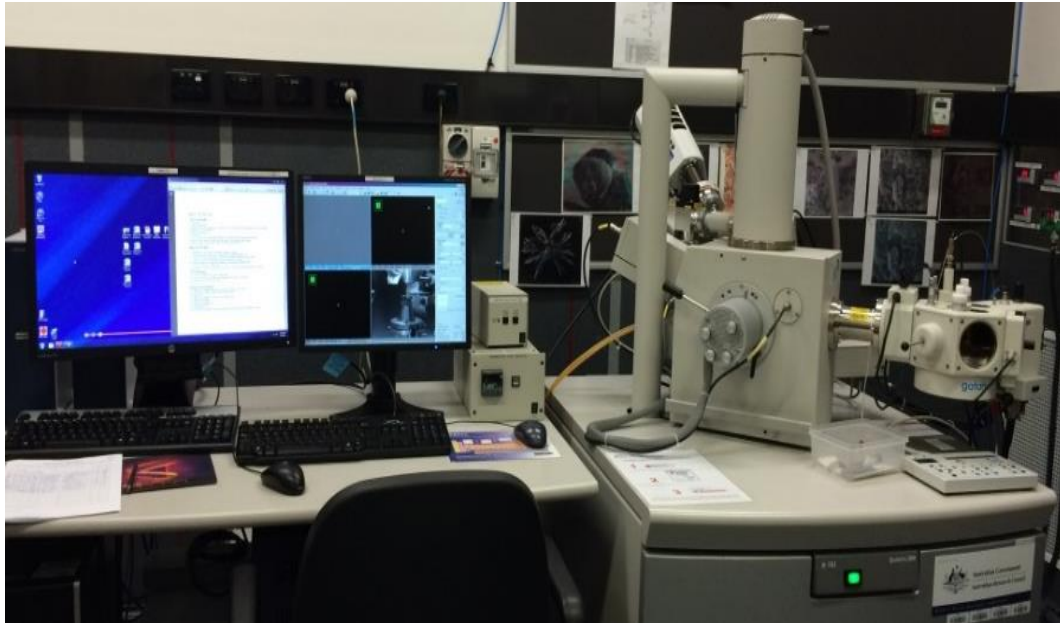
Figure 3.2 SEM FEI Quanta 200 equipped with EDX instrument
