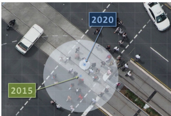
Figure 3. The effect of Australia's continental drift of around 7 cm north-east each year when comparing positions from the static 1994 Australian datum GDA94 in 2015 and then in 2020.
