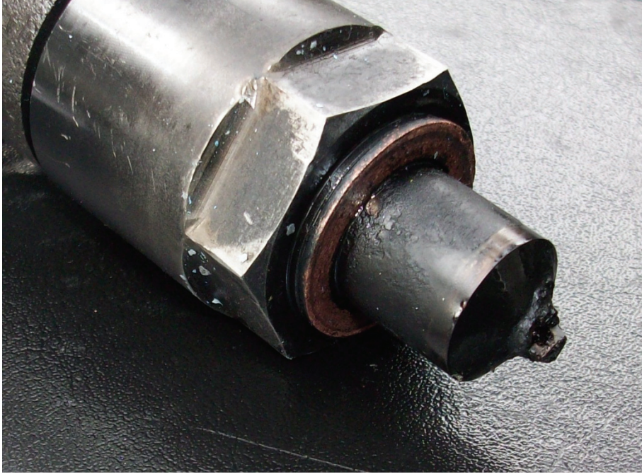
Figure 8.7 Injector nozzle damage caused by high temperature
