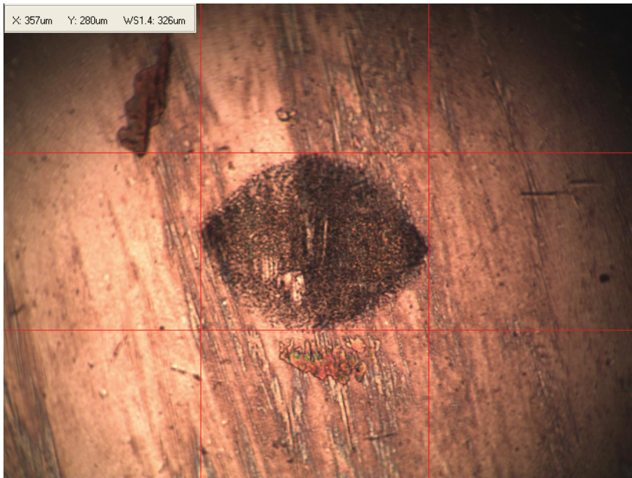
Figure 6.4 Wear scar captured by digital microscope; ULSD at 60°C
