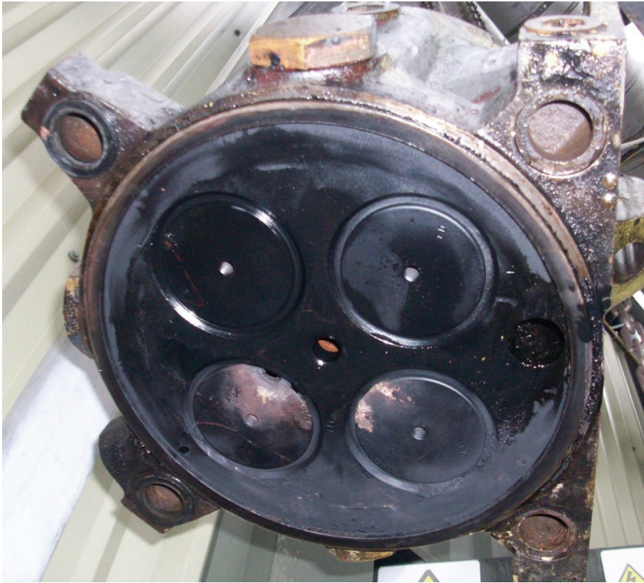
Figure 8.9 Ruston 6AR cylinder head - valve damage visible
