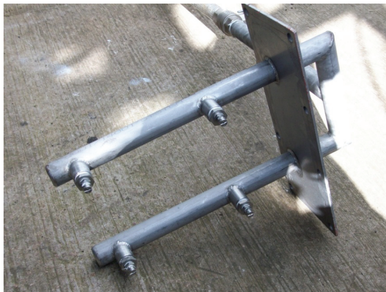
Figure 4.9 Water injecting nozzles
