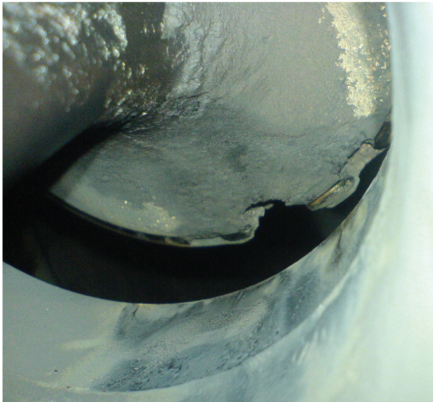
Figure 8.8 Burned exhaust valve
