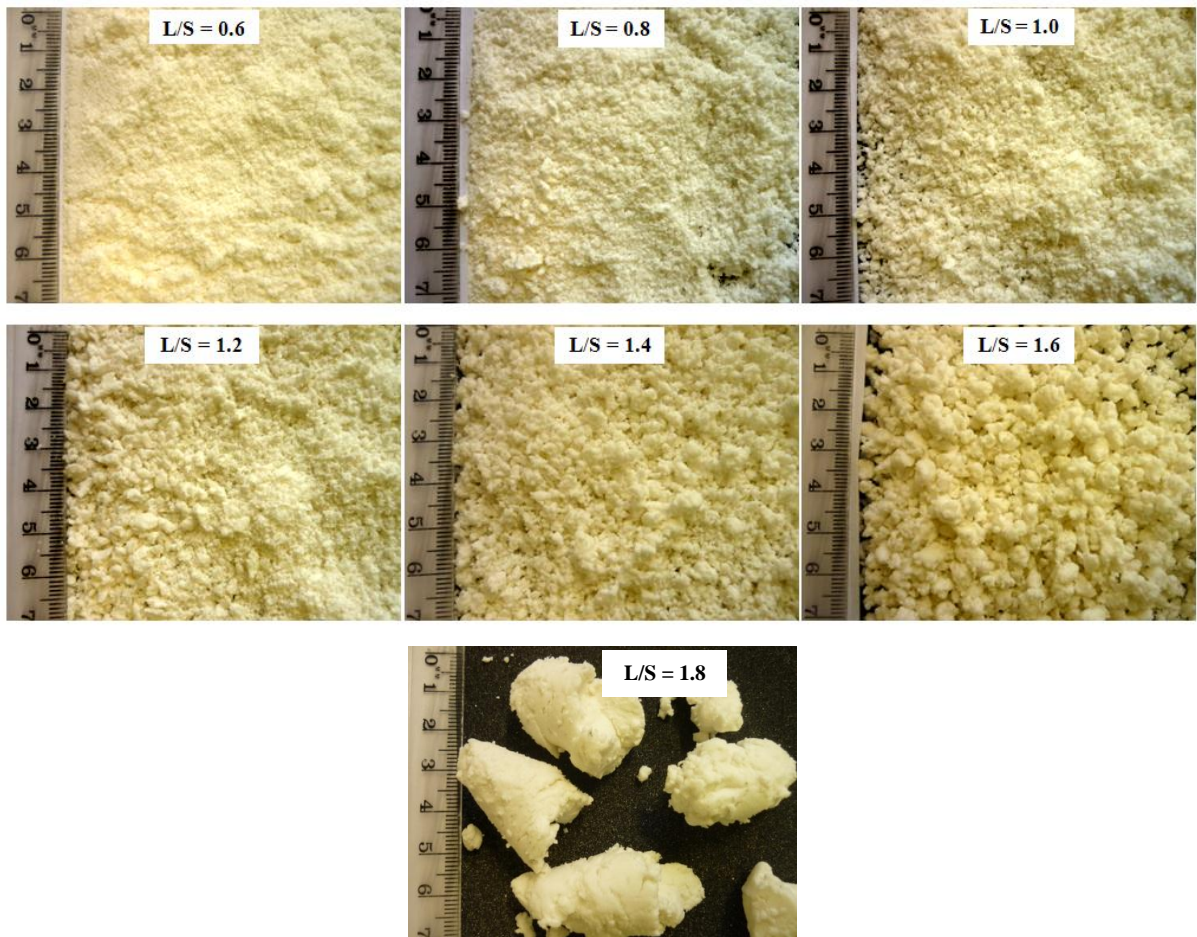
Figure 4-4: Granules produced by TSE at 500 rpm using various liquid to solid ratio (dimension in cm)
