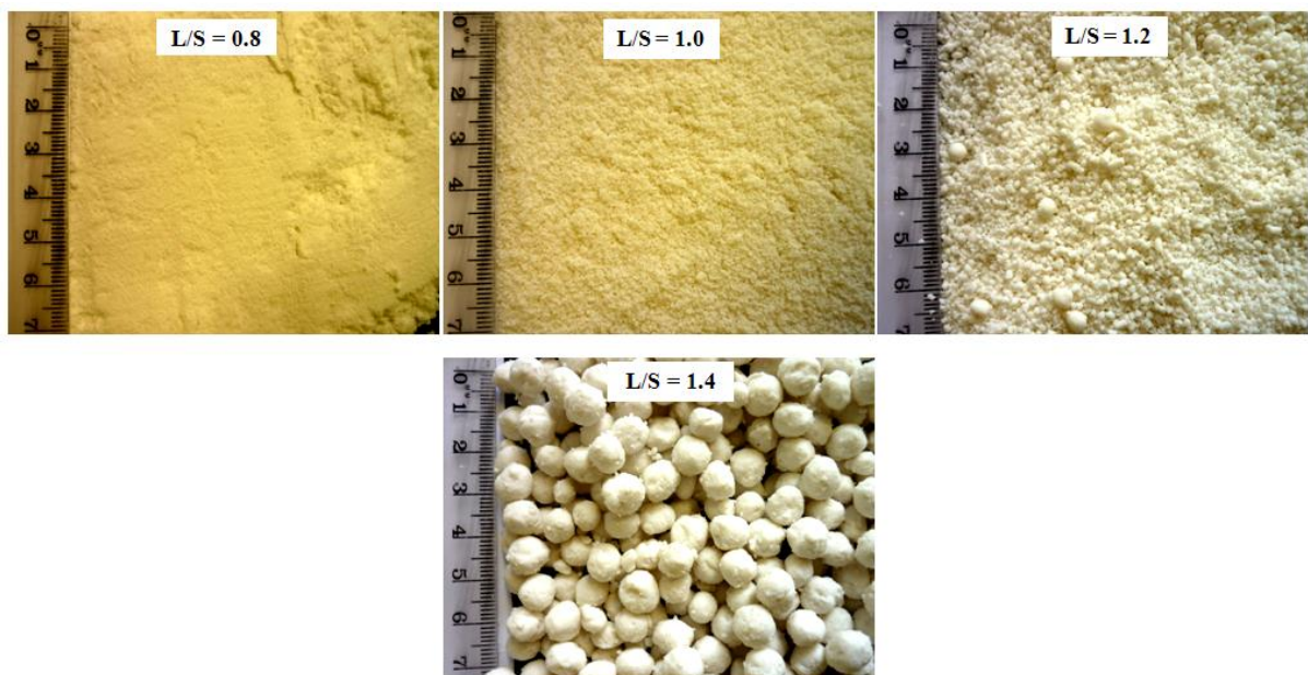
Figure 4-5: Granules produced by HSM at 600 rpm using various liquid to solid ratio (dimension in cm)
