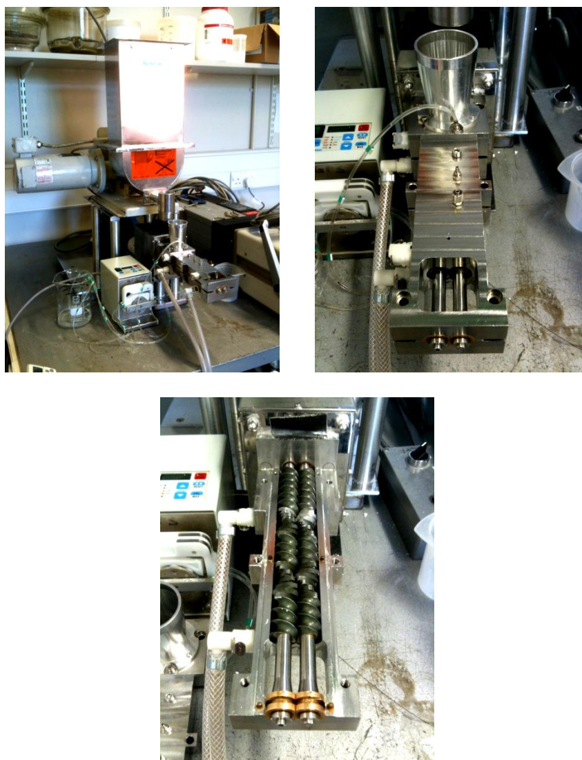
Figure 3-5: Twin screw granulator used for PEPT study provided by GEA Pharma System
