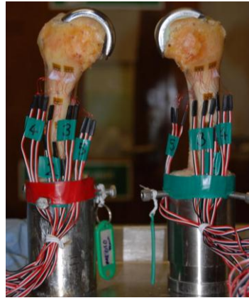
Figure 46 - A paired set of femoral bone constructs (from the same donor) with strain gauges carefully positioned in similar locations.
