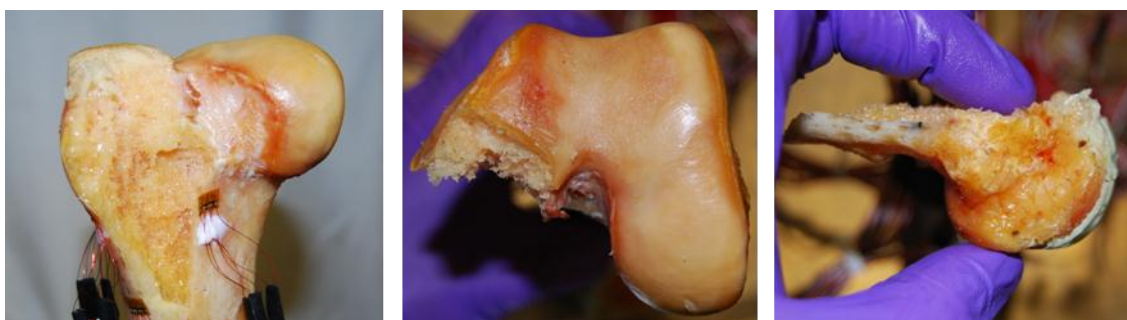
Figure 72 - Implanted femur which failed at the anterior resection.
