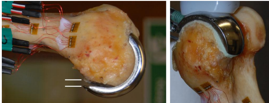
Figure 69 - Overcut femur posterior (left) and cemented to fill the gap (right). Since the femur posterior is hidden from view during arthroplasty, it is difficult to achieve a perfect resection.
