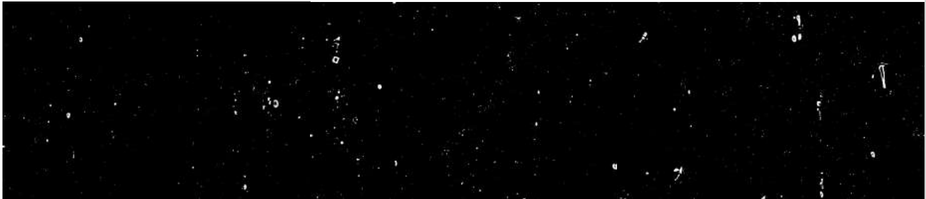
Figure 63 – Microstructure and precipitate count of 600°C 192h heated sample
