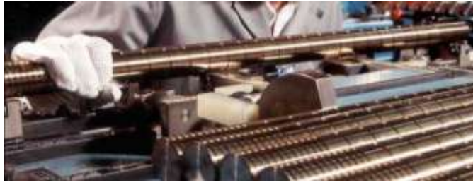
a) MAGNOX fuel: natural uranium metal 'billet', adapted from BNFL Oxide Fuel Brochure [32]
