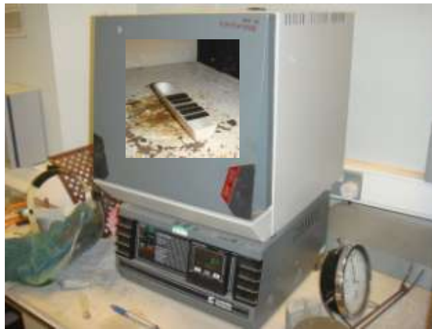
c) Heat treatment (inset: sample on crucible inside the oven)
