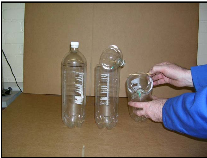
Figure 2.1: Construction of bottle traps for amphibian sampling. On the left is the drinks bottle from which the trap is constructed. In the centre, the top section has been removed and the hinge fitted to one side of the inverted top section. On the right is the completed trap with the cocktail stick inserted to act as a lock.
