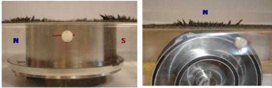
Fig. 5. Illustration of the manufactured prototype magnetic scroll air motor (N: North Pole; S: South Pole) [19]
