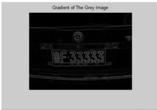
Figure 3. The gradient of the grey image
