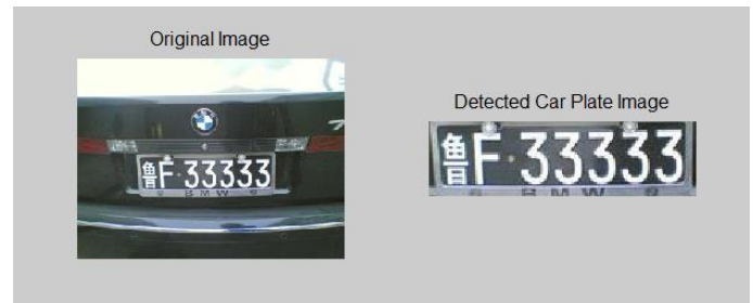
Figure 14. The detected car license plate-1
