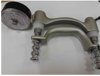
Fig. 2: Saehan hydraulic hand dynamometer used to measure grip strength[25].
