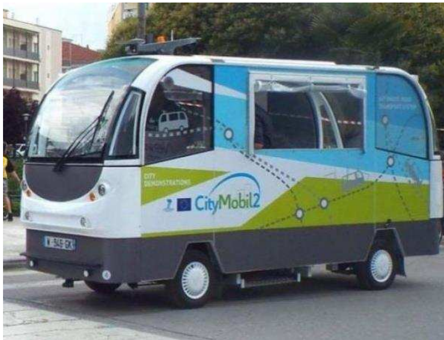
58 Figure 1: An example of one the CityMobil2 ARTS Vehicles (designed by Robosoft)
