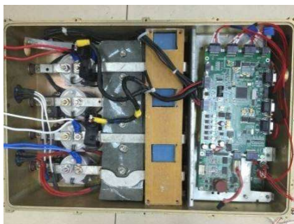
Fig.15 Si-IGBT based power converter for PMSM direct drive system.
