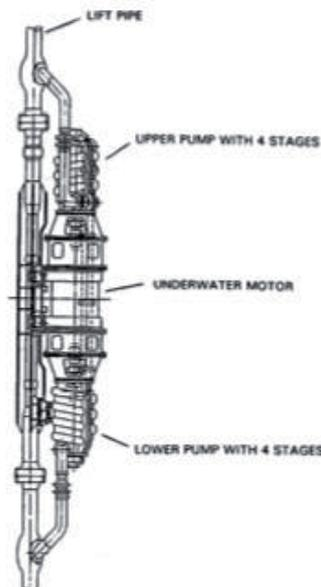
**Figure 32:** Deep-submersible pump with underwater electric motor (TRAM 1991)
