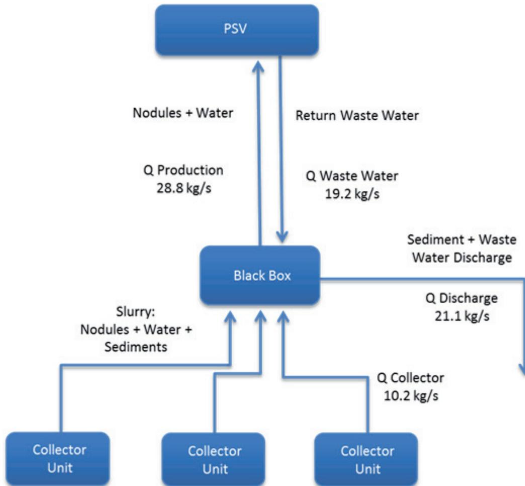
**Figure 43:** Mass flow rate of the whole single production system
