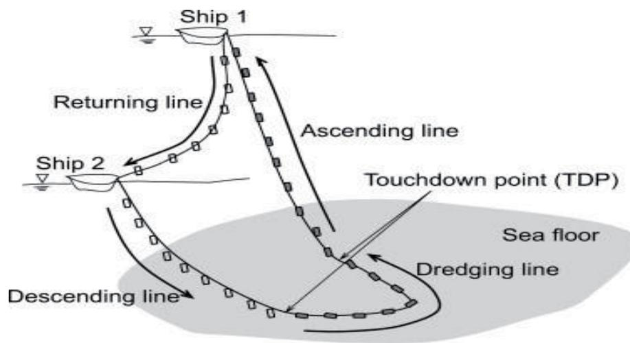
**Figure 30:** The line bucket system in operation (Brockett 1999)
