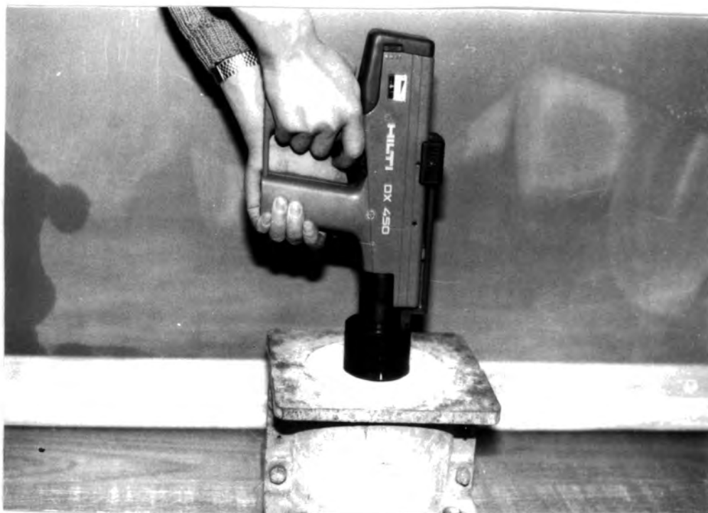
Figure 3.3 Experimental arrangement for penetration test
