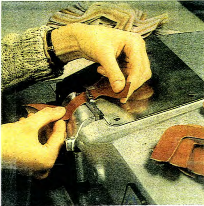
Fig. 1.3 The manual skiving operation ( by permission BUSM Ltd ).
