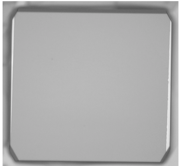
Fig. 2: Typical 3C-SiC layer grown on 0.2 mm x 0.2 mm SD-free mesa on Sample B following oxidation to reveal SF defects.
