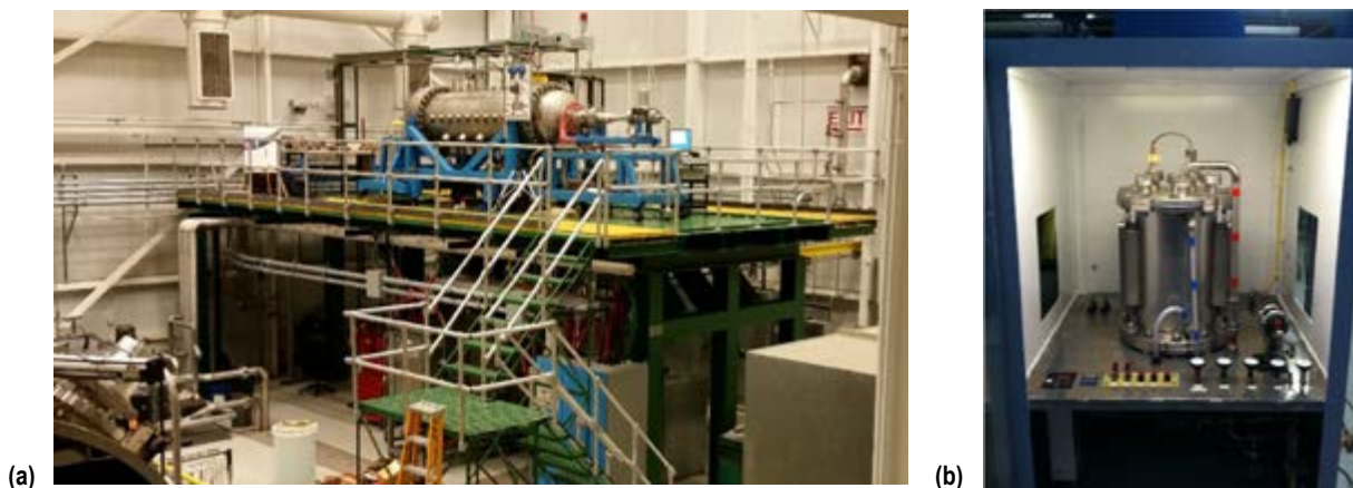
Figure 3: MSFC test facilities: (a) Nuclear Thermal Rocket Element Environmental Test System (NTREES) and (b) Compact Fuel Element Environmental Test (CFEET) System.
