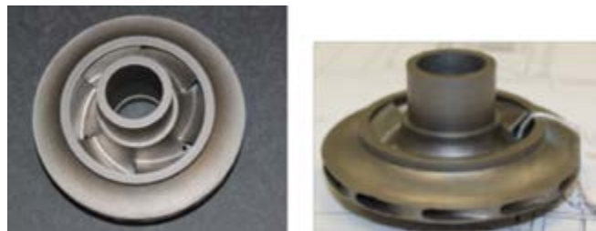
Figure 2. SLM Ti6-4 manufactured turbopump impeller.
