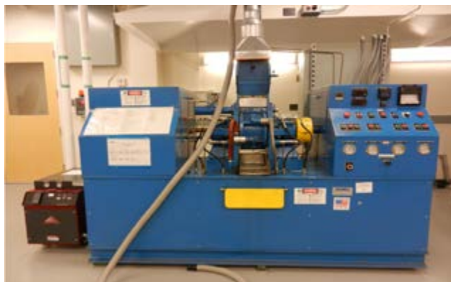
Rubber Lab mixer and control system.
