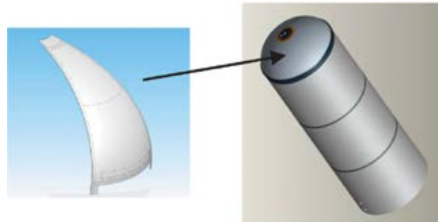
Figure 1: Gore panels are welded together to form the dome ends of SLS cryogenic tanks.
