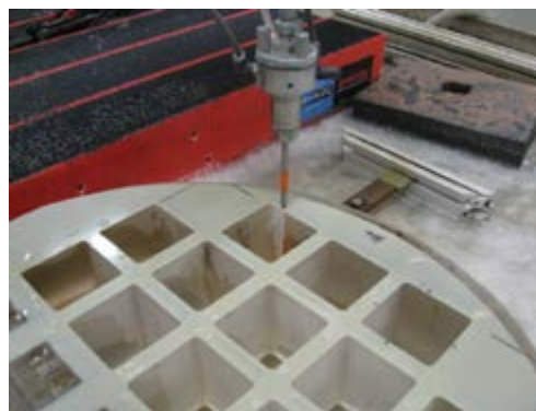
MOR specimens in abrasive waterjet cutting.
