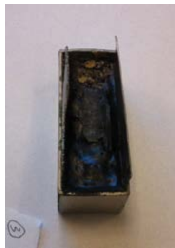
Lunar regolith sintered brick.
