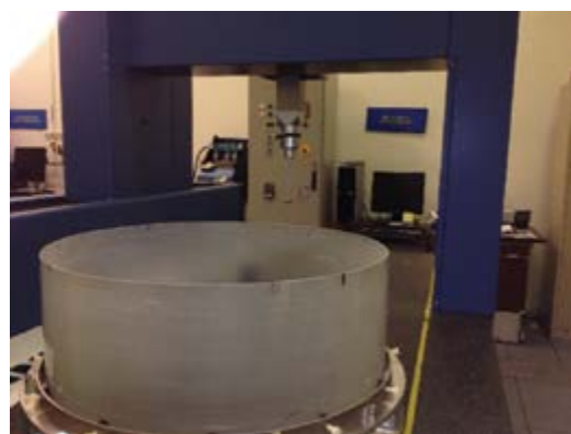
Figure 2: Thick glass shell on coordinate measuring machine.
