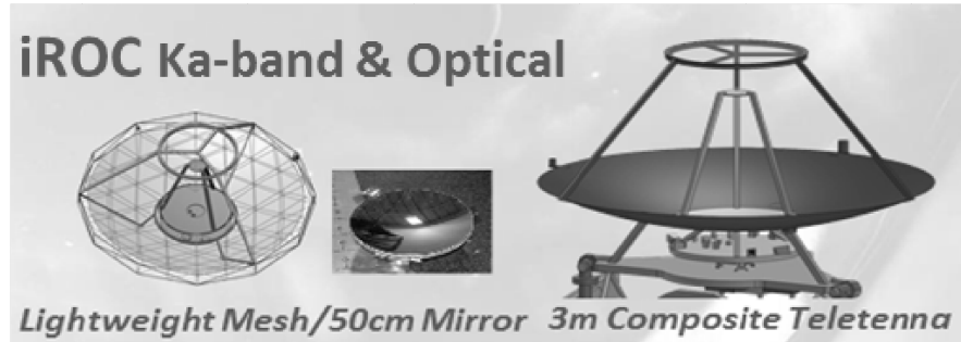
Figure 4. The integrated Radio and Optical Communications (iROC) terminal, a technology investigation to merge Ka-band RF and 1550 nm optical communications within the same size, weight, and power (SWaP) of today's current RF systems. (Figure courtesy of Dr. Daniel Raible, NASA GRC).
