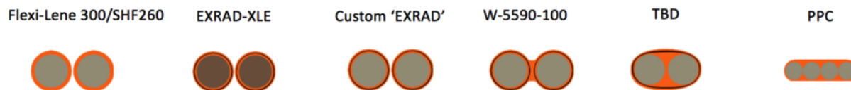
Figure 3. Cable selection options, all assuming an equivalent 4AWG and sized based on SAE AS50991. The PPC wire on the right was chosen for the final design.
