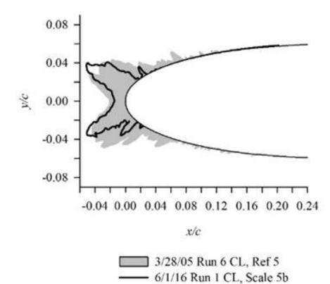
$MVD_5 = 26.8 \mu m$ ,  $LWC_5 = 0.56 \text{ g/m}^3$ ,  $t_5 = 8.5 \text{ min}$  $MVD_{5h} = 19.3 \mu m$ ,  $LWC_{5h} = 0.37 g/m^3$ ,  $t_{5h} = 14 min$
