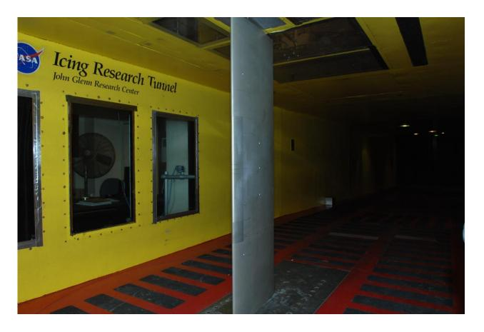
21-in chord NACA 0012 model, full span
