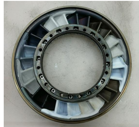
Figure 15. Turbine nozzle ring with candidate coatings
