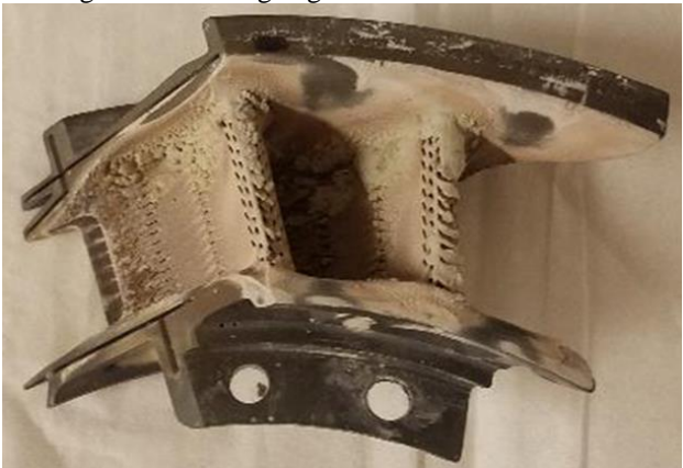
Figure 17. Reference nozzle with the OEM applied CoDEP coating
