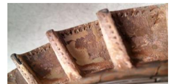
Typical build-up on blade
