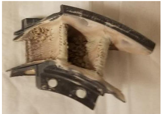
Figure 19. ARL-NASA-01 (8YSZ applied with SPPS) post-test picture
