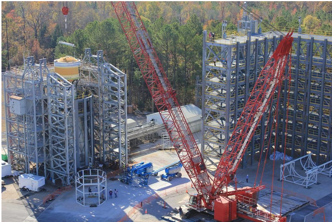
Fig. 5. A structural test article of the Interim Cryogenic Test Article is installed for testing.
