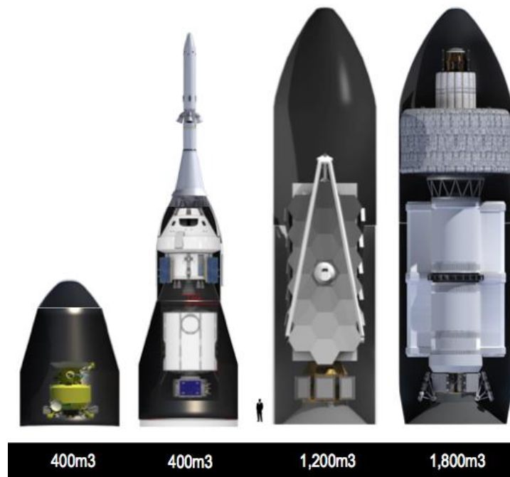
Fig. 7. Fairing options for evolved configurations of SLS.
