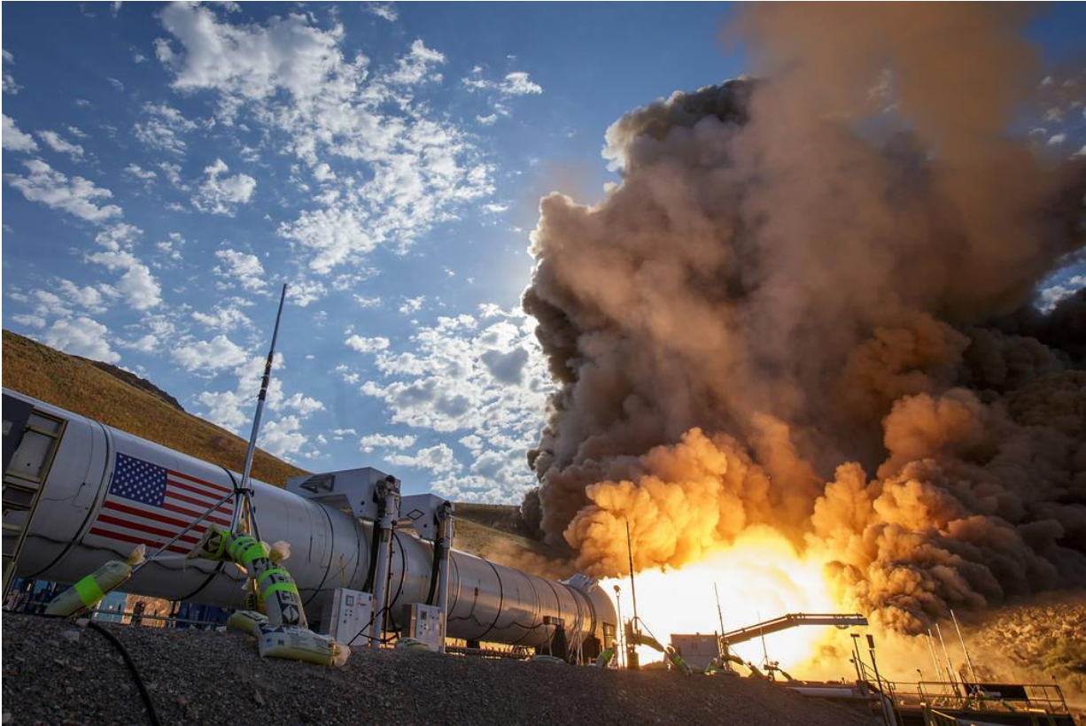
Fig. 4. Qualification Motor-2 test of the SLS solid rocket booster.
