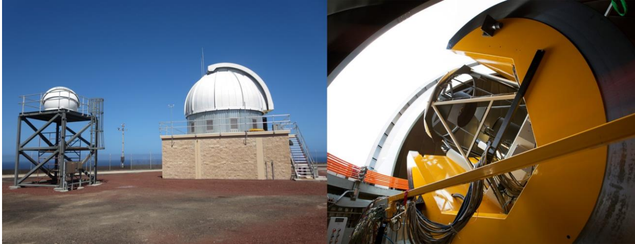
Fig. 1: Left: The ES-MCAT Observatory is comprised of the 1.3-m ES-MCAT telescope (larger building on the right) and a tower platform (left) that will house a 0.4-m Officina Stellare telescope by 2018 [2]. The weather mast can be seen between the two telescopes. Right: The 1.3-m ES-MCAT (a.k.a. MCAT) telescope, demonstrating the horseshoe mount that allows it to track smoothly through the zenith at Ascension's low latitude site.
