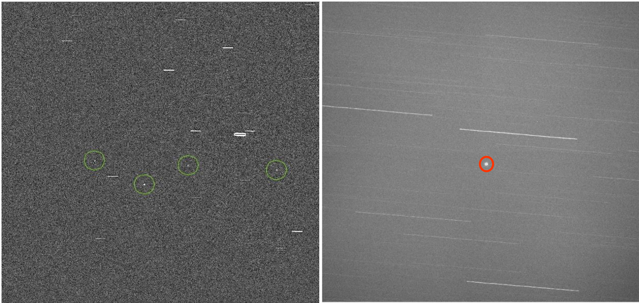
Fig. 4: ( LEFT ) Images taken in GEO mode or RT will result in streaks of equal length and orientation for the stars, while RSOs in GEO (green circles) will appear point-source. Four RSOs are evident. (North is up, east is left) ( RIGHT ) An image taken at LEO following an RSO's TLE demonstrates much longer star trails for the faster moving LEO object (red circle).
