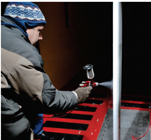
Figure 1. Painting an Ice Accretion in the Icing Research Tunnel at NASA Glenn
