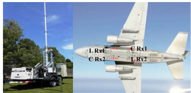
Figure 1. Ground Station and Antenna Tower on Transportable Trailer S Trailer and the NASA GRC S-3B Viking Test Aircraft with Receive Antenna Locations
