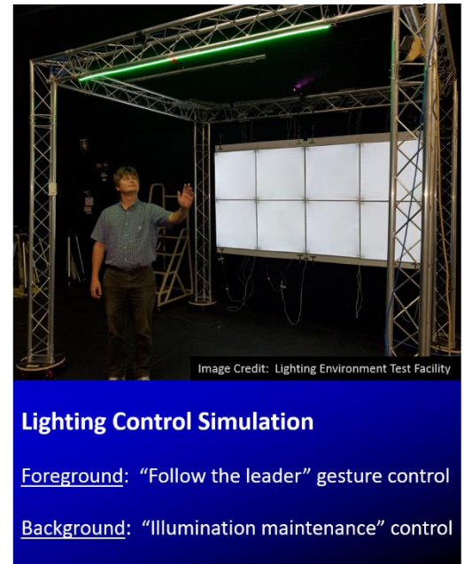
Figure 3: Lighting Control Simulation
