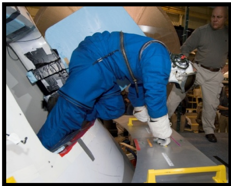
Orion emergency pad egress
