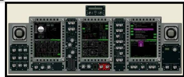
Human factors input resulted in increased in-line and cross-cockpit viewability, improved reach and access to controls, better labeling and use of LEDs, and improved organization and placement of controls.
