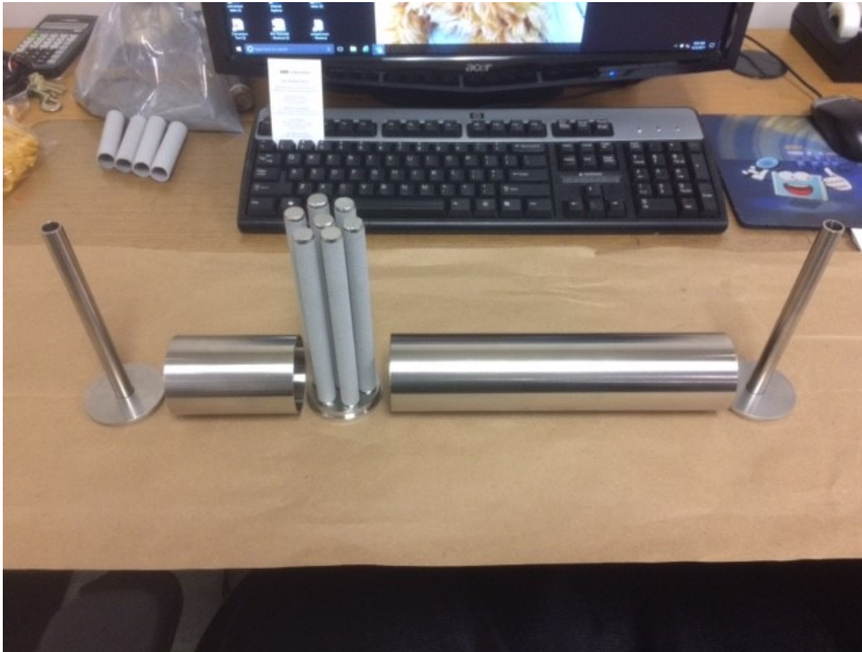
Third generation porous metal filter before welded assembling
