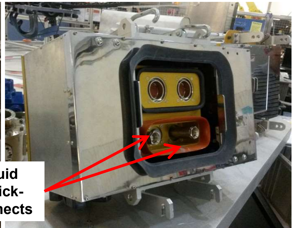
Active half manually latched to passive half for fluid transfer
