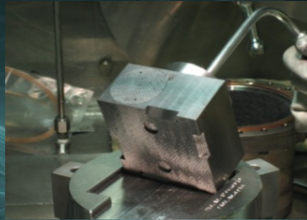
General Purpose Heat Source Module
