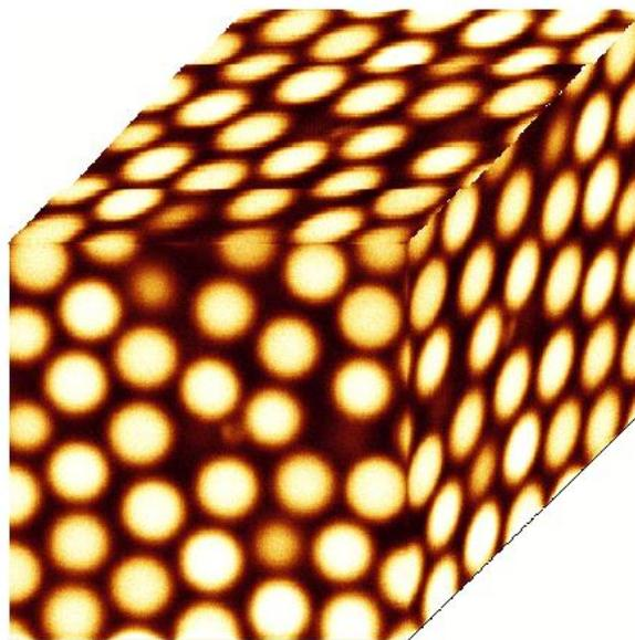
**3D image is built out of 2D XY sections while stepping through Z axis.**
