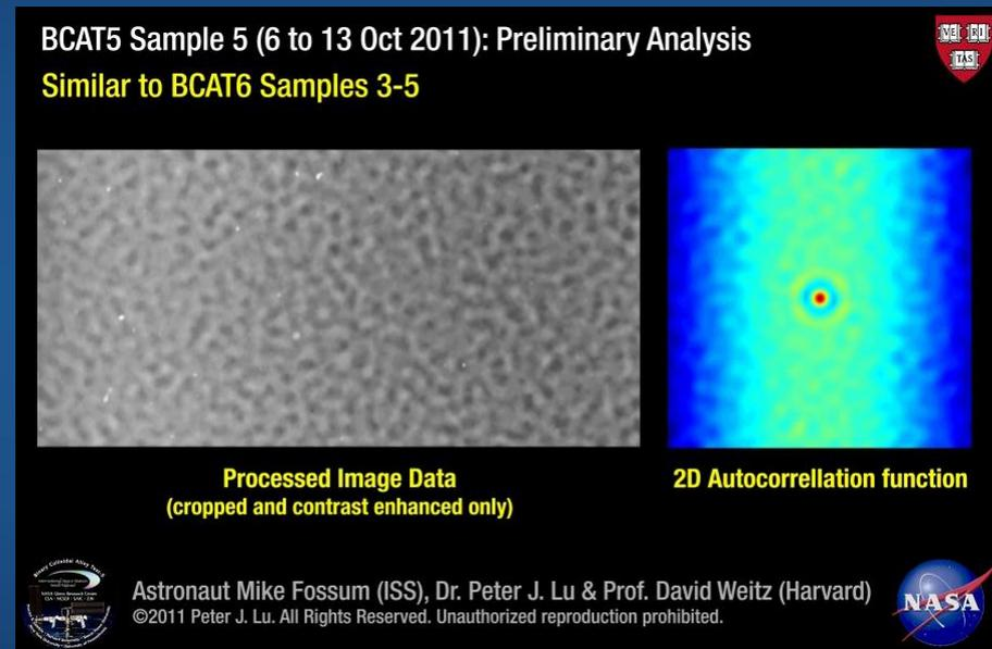
Phase separation no longer has a top or bottom in microgravity. Coarsening can be observed over an extended period of days to months, as seen in the above movies. Please click on images to play movies.
