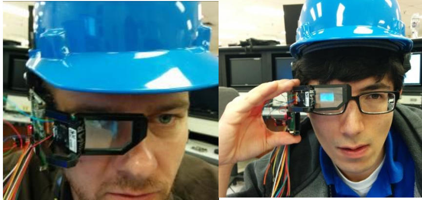
Figure 12: Early version collimator usability tests (optical engine: OE-32 Optical engine with 720p resolution (1366x768). I believe power was about 3w, ~35 degree FOV, 4000 nit brightness) with and without glasses using temporal bone (side) position and hardhat as the subsystems wearability support. Tests concluded that side position of the projector will never comply with individual anthropometry and ergonomics requirements.
