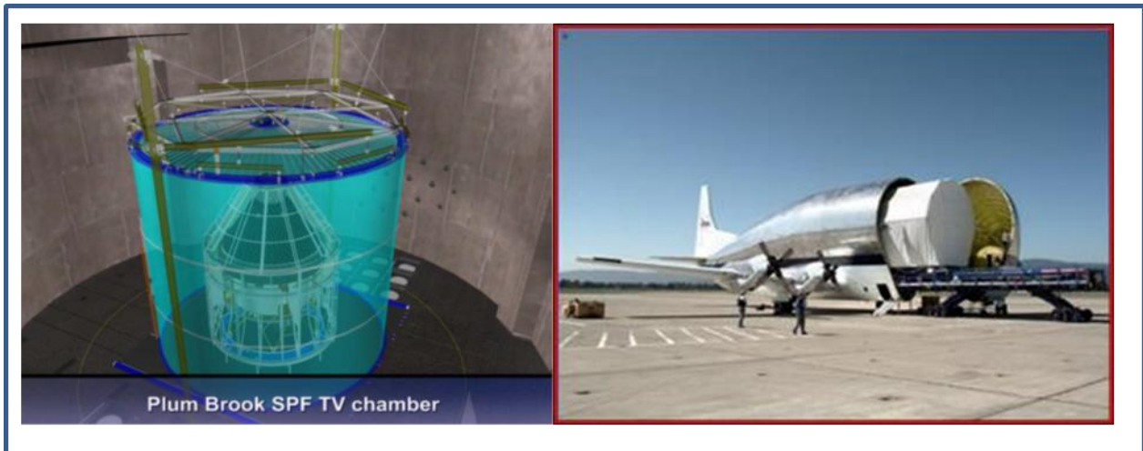
Figure-8- EM-1 Test configuration CAD Model Located in PBS and NASA Super Guppy Transporter
