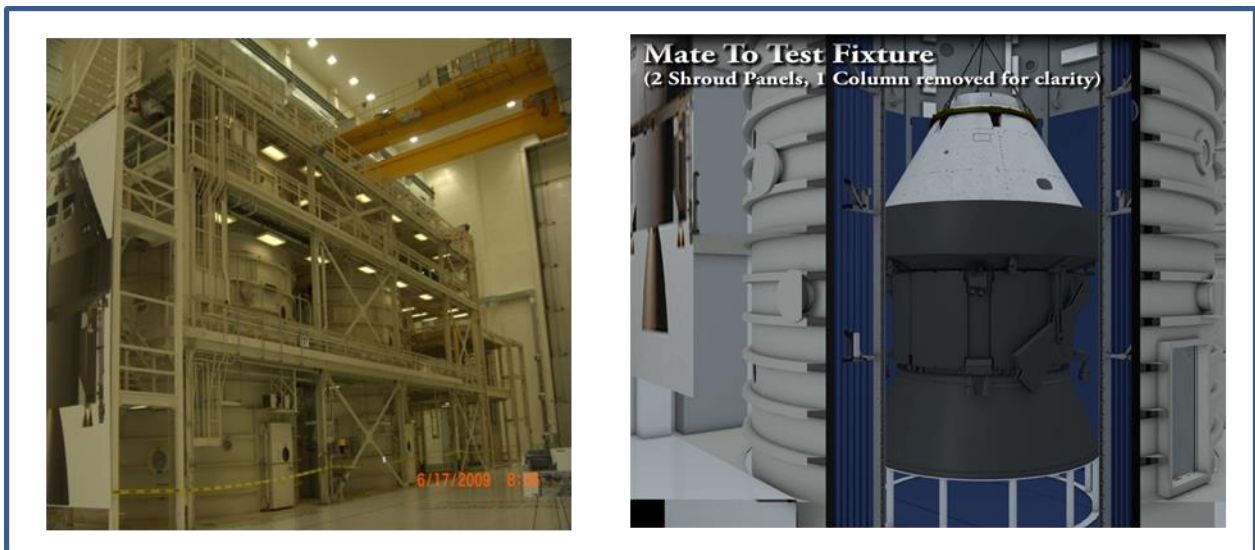
Figure-10- O&C Altitude Chambers in the High Bay with CAD Model Installed in Test Chamber
