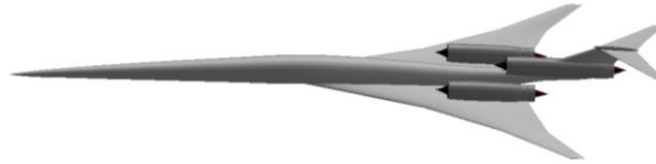
Figure 3. Solid model of notional supersonic business trijet.
