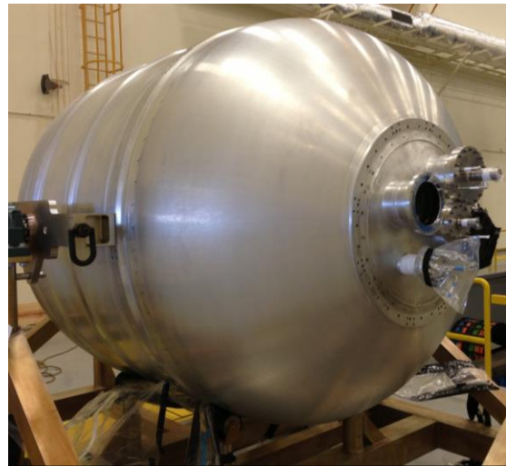
Figure 1: CPST EDU tank during fabrication at Marshall Space Flight Center. External view of tank without MLI or foam.
