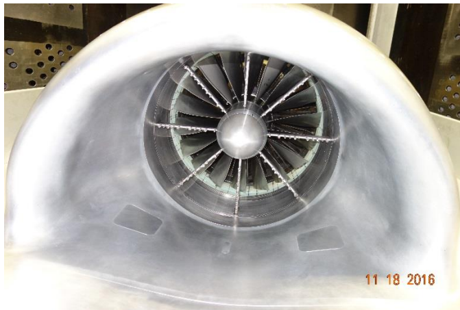
Figure 4. Front View of Propulsor with AIP Rakes Installed
