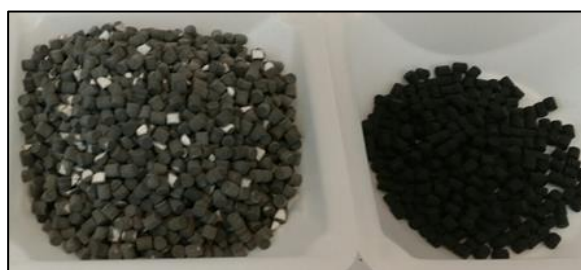
Figure 18. The spent catalyst (left) was removed from the Sabatier reactor after it no longer performed as expected. It is much lighter in appearance and has many broken pellets compared to unused catalyst (right).
