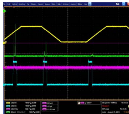
Figure 6. An oscilloscope record for the LTC and WCU synchronization using the Q-switch enable signal (blue). The ramp signal (yellow) is used for injection seeding by the ramp-and-fire method. Energy monitor (red) and target return (green) signals are digitized and recorded using the IPDA data acquisition system.
