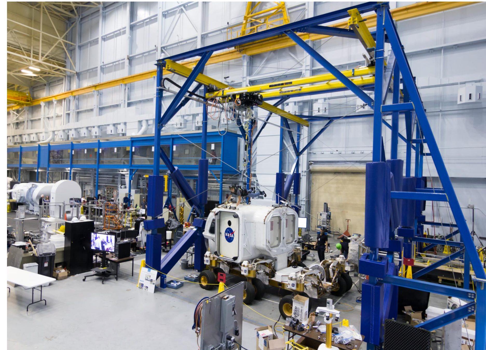
Active Response Gravity Offload System (ARGOS) at JSC
