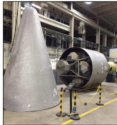
Fig. 7. Nosecone removal and staging after the test article’s arrival at NASA JSC. Note sample payload attachments that show how a Titan IIIC Transtage was used to put satellites in a GEO orbit.
