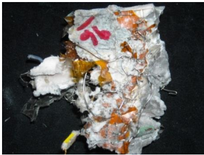
Fig.22. Composite fragment from an impact experiment based on a 1960s era Transit satellite. The color-color plot matched the closest with the observed SSN 3432 Titan Transtage fragment.
