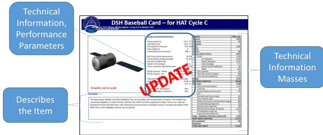
Figure 5. An example traditional space system baseball card focused on technical information. 52 Technical, performance information usually emphasizes mass, plus other characteristics like mission duration or crew capacity. Were this a propulsion stage there would be an emphasis on masses and type of propellant, plus other characteristics like engine thrust or number of engines.
